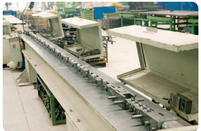
Pre-stressing after final assembly
