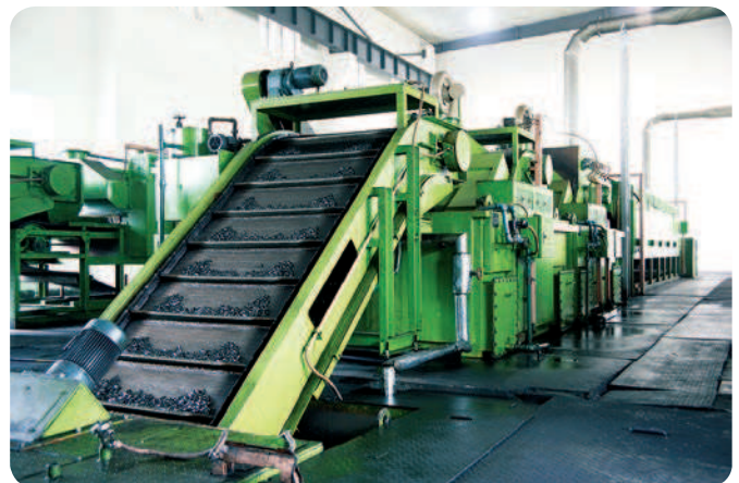
Conveyor furnace line used for roller and bushing heat treatment, e.g. carbon-nitriding
